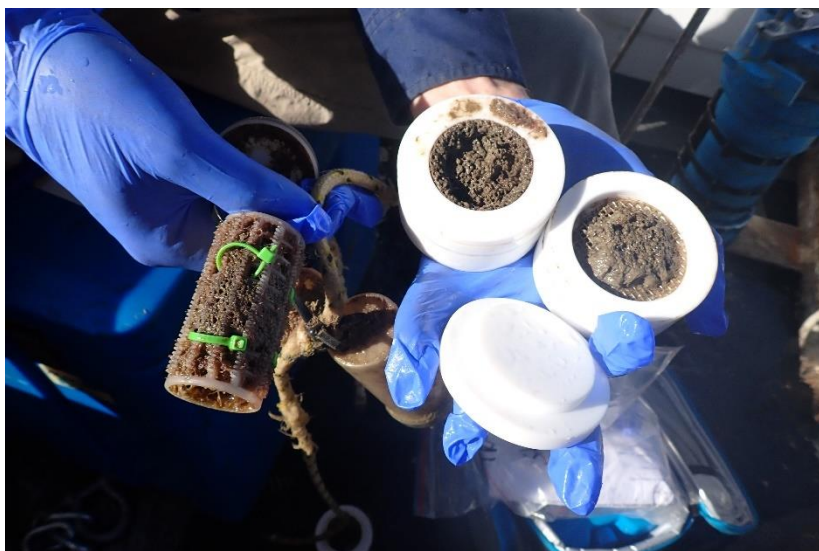
Figure 2-2. Pesticide monitoring passive samplers such as these were retrieved from Aquila Island (MKY_CAM1) over the reporting period (Table 2-5). Note: biological growth on the samplers.
