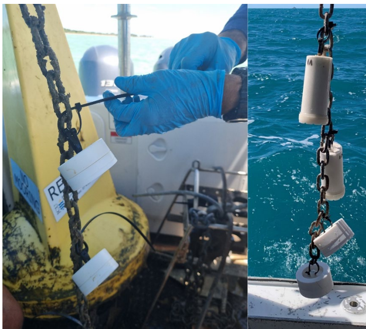
Figure 2.2. Pesticide monitoring passive samplers were deployed at Aquila Island (MKY_CAM1) throughout the wet season. Empore disk (ED) samplers and passive flow monitors (PFM) pictured being prepared for deployment.
