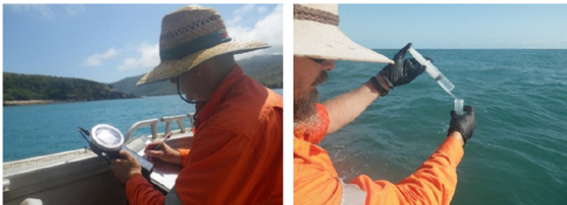
Fig 5: TropWATER staff measuring and recording water quality parameters with a mutiprobe (left) and collecting a water sample for laboratory analysis (right) during water quality sampling trips (2019).
