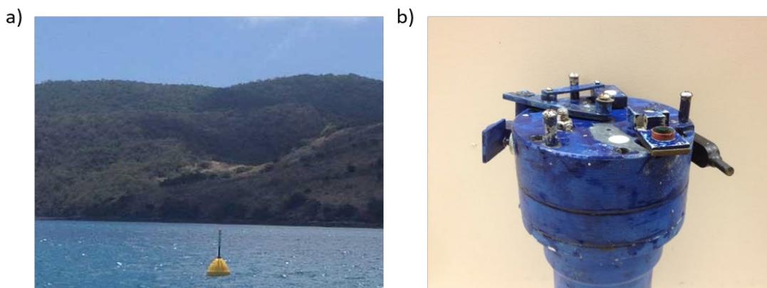
**Figure 2.2** Example coastal multiparameter water quality instrument: a) site navigation beacon for safety and instrument retrieval; b) instrument showing sensors and wiping mechanisms
