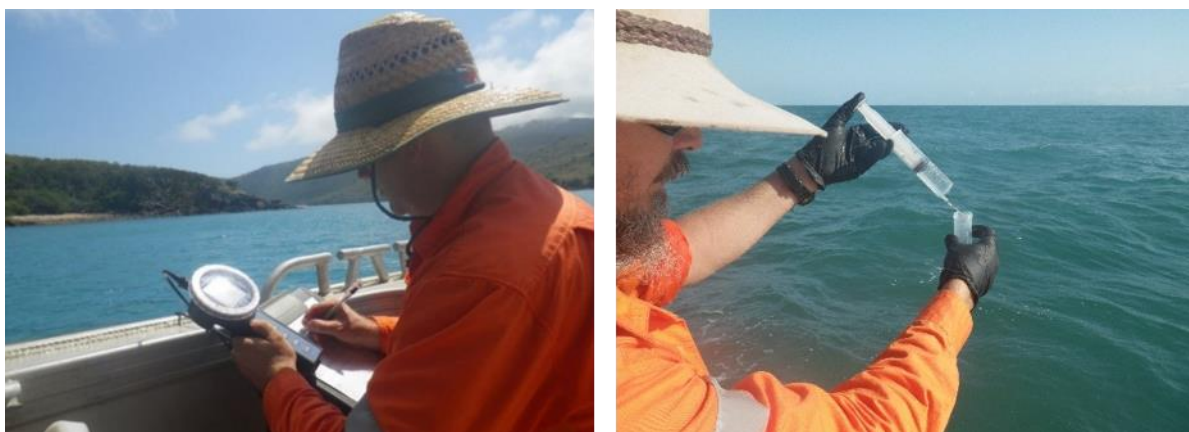
Figure 2.1 TropWATER staff measuring and recording water quality parameters with a multiprobe (left) and collecting a water sample for laboratory analysis (right) during water quality sampling trips.
