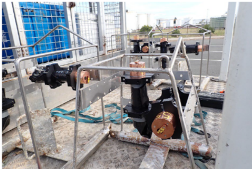
Fig 4: Water quality loggers ready for deployment to the seabed. The horizontally orientated logger is an NTU-LPT turbidity logger, and the vertically orientated logger is a MS9-LPT multispectral light logger manufactured by Insitu Marine Optics (2022).
