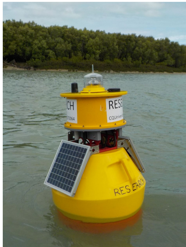
Figure 1: YSI EXO2 sonde and EMM65 monitoring buoy, deployed at Carmila Creek estuary in January 2022.
