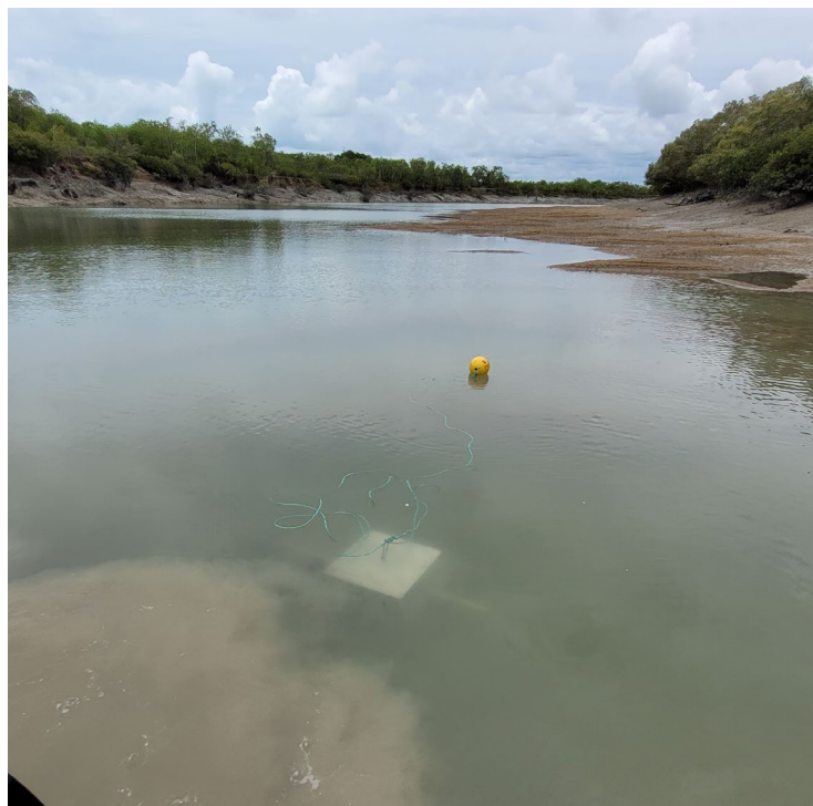
Figure 1: A baited remote underwater video station (BRUVS) deployed at Carmila Creek estuary in January 2022.
